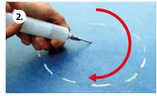
Inject a small amount of Eurocol Linoleum Doctor into the bubble. During injection, move the syringe circularly around the drill hole.
