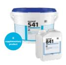
Rollable bonding dispersion which provides full area anti-slip coat after drying. For fixation and for multiple, removable installation of heavy, self-laying, form stable carpet tiles with bitumen/vinyl or PU heavy coating (> 4 kg/m²) on standard absorbent or non-absorbent subfloors. For electrically conductive (EC) installation, mix 10 parts of 541 Eurofix Anti-Slip with 3,5 parts of 841 Europrimer EC.
